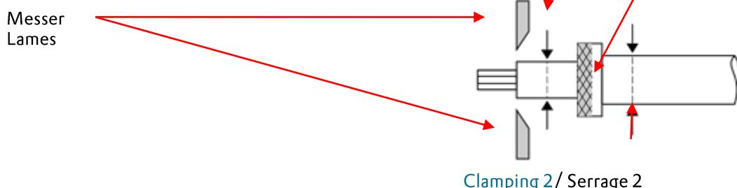
The clamping jaws 1 (inside) engage in front of the support ring, the clamping jaws 2 (outside) behind them.
